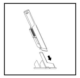
Charge the unit by sliding it into the charging base nozzle-first.
