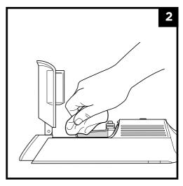
2. Wipe the screen inside the **Dust Cup** lightly with a dry cloth to remove dust and dirt.
