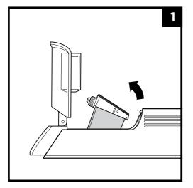
1. With the dust cup removed and the power off, pinch both sides of the filter housing and pivot it upward to access the filter.
