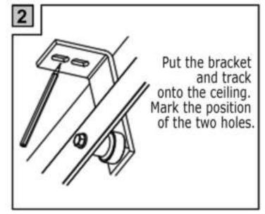
Drill holes on the marked position.
