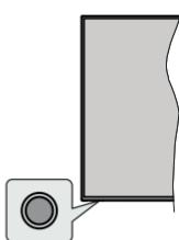
The control button allows you to control the Quick Standby-On functions of the TV.
