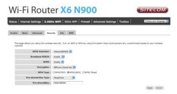
Wi-Fi Protected Access (WPA) is an advanced security standard. You can use a preshared key to authenticate wireless stations and encrypt data during communication. It uses TKIP or CCMP (AES) to change the encryption key frequently, so the encryption key is not easy to be cracked by hackers. This is the best security available.
