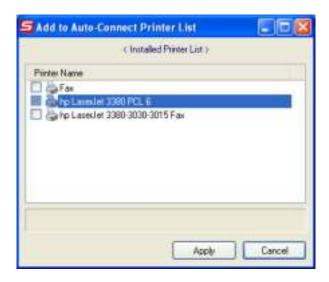
• Choose the desired printer. The desired printer must be the Windows printer (this is a logical printer) that matches the printer attached on the MFP server (this is a physical printer). Then click the "**Apply**" button.
