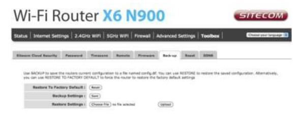
Use the "Backup" tool to save the current configuration to a file named "config.bin" on your PC. You can then use the "Restore" tool to restore the saved configuration to the router. Alternatively, you can use the "Restore to Factory Defaults" tool to force the router to perform a power reset and restore the original factory settings.
