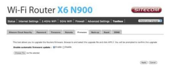
**Enable automatic firmware update**: When enabled the router will periodically check if a new firmware is available. If a new firmware is detected the router will give a notification.
