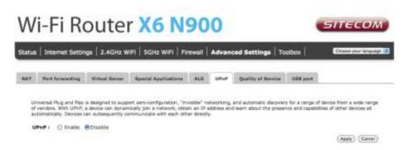
**UPnP Feature**: You can enable or Disable the UPnP feature here. After you enable the UPnP feature, all client systems that support UPnP, like Windows XP, can discover this router automatically and access the Internet through this router without having to configure anything. The NAT Traversal function provided by UPnP can let applications that support UPnP connect to the internet without having to configure the virtual server sections.
