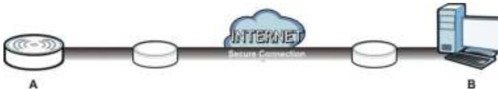
Figure 78 SSH Communication Over the WAN Example
