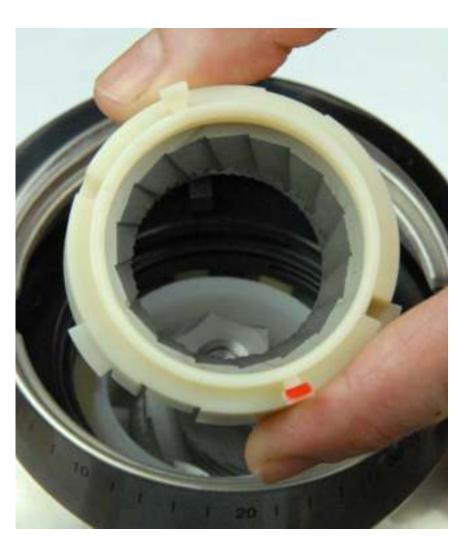
far as it will go. Replace the burr by lining up the red tab on the burr with the rectangular cutout on the black adjustment ring. Wiggle and push down firmly on the ring burr to ensure that it seats properly. After replacing the burr, replace the silicone seal by lining up the two slots in the silicone seal with the small tabs on the top of the ring burr and slide the seal onto the ring burr.
