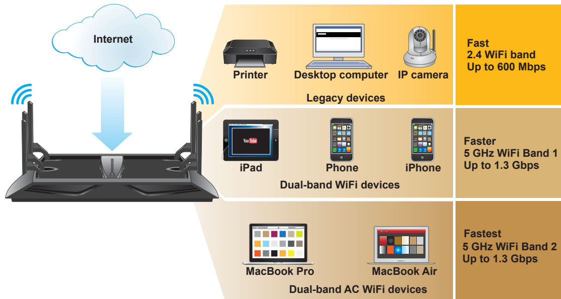
Figure 10. Load balancing in a tri-band WiFi network
