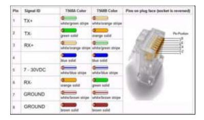
Though the device can be powered over Ethernet port it is not compliant with IEEE 802.3af-2003 standard. Powering RUT9xx from IEEE 802.3af-2003 power supply **will damage the device** as it is not rated for input voltages of PoE standard.
