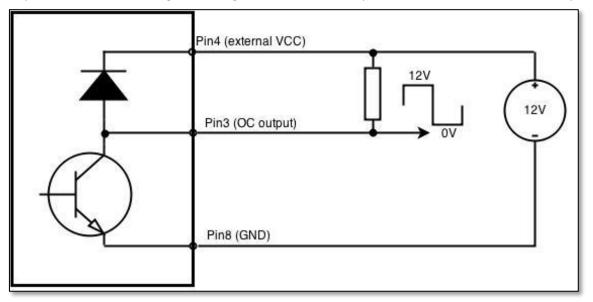
Output can be also used to generate signals with desired amplitude. Resistor could be for example 4.7kΩ.
