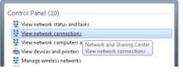
4. Then right click on your wireless device that you use to connect to other access points (It is the one with the name "Wireless Network Connection" and has signal bars on its icon).
