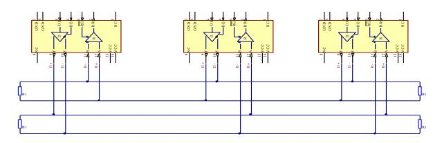
Example 2-wire network electrical connection: to enable 2-wire RS-485 configuration in Teltonika router, you need to connect D\_P to R\_P and D\_N to R\_N at the device RS-485 socket. Termination resistors are placed at each cable end.
