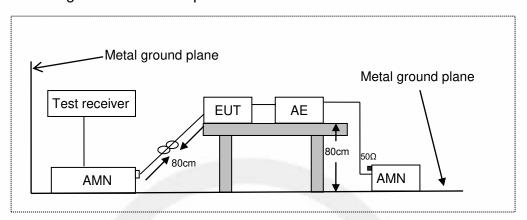
AMN: Artificial Mains Network AE: Associated equipment EUT: Equipment under test
