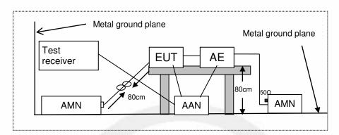
AMN: Artificial mains network AE: Associated equipment EUT: Equipment under test
