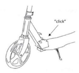
By opening the quick release, you can adjust the steering to a comfortable height. Make sure the knob snaps in to a hole in the steering column. After adjustment, close the quick release.
