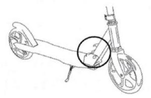
By pulling the trigger, you can unfold the scooter.
