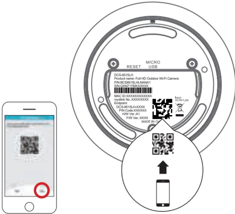
When prompted, select "Yes" to scan the QR code on the bottom of the camera, then continue to follow the onscreen instructions to complete the setup process.
