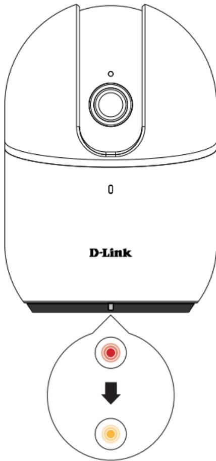
Once the camera has powered up, it will rotate left and right, up and down to calibrate itself. Wait until the LED at the front changes from red to blinking orange.
