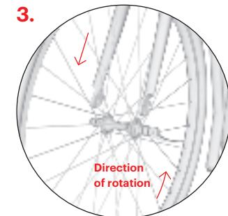
Insert the wheel into the front fork so it is exactly in the middle. **Caution:** When inserting the wheel, ensure that the tyre pattern points in the direction of rotation when the scooter is rolling forwards (on some tyres see direction arrow on the side).
