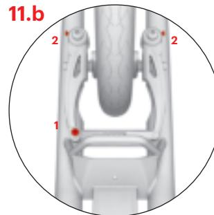
Check that the brake pads move away from the rim sufficiently (1–2 mm) when the brake lever is re-released. The distance of the brake pads can be adjusted by tightening or loosening the brake cable anchor bolt (1). If the brake pads come into contact with the rim while the wheel spins, adjust the spacing of the brake arms symmetrically with the tensioning bolts (2).
