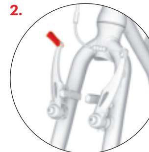
First, check that the front fork of the scooter is aligned correctly (the V-brake shoulders should be pointing forwards towards the front of the scooter), then release the brake jaws by rotating the lever.
