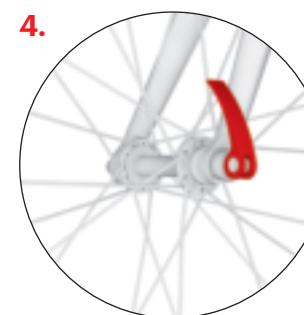
Tighten the adjustment nut of the quick release mechanism to the correct position. When it is in the correct position you will feel a noticeable resistance just before you close the mechanism completely. Close the quick release lever in a position where it does not touch the fork and simultaneously it cannot be opened accidentally while riding.
