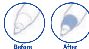
Leap™ pH Probe bridge before and stained after preconditioning in soil. This is normal.
