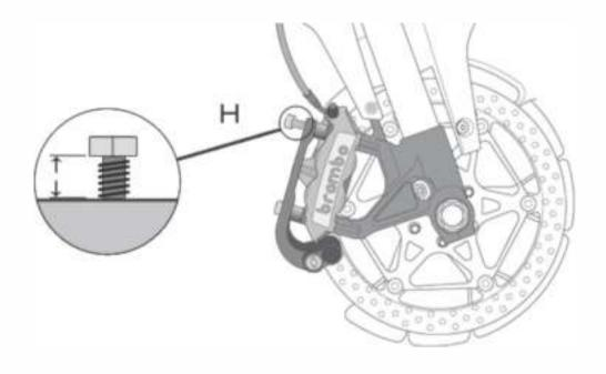
**NOTE 1:** If proper installation requires a thread length in between 80mm and 90mm, the included 5mm shims (X) can be used between the bolt and the RoadLoK body. Combining the 5mm shim with the 90mm bolt will result in an effective 85mm thread length, which may be more appropriate for some models.
