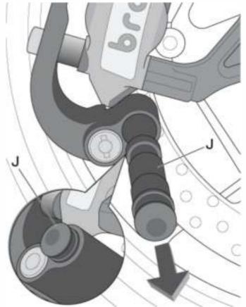
7. Insert the pin (I) into the hole where the black plug was removed. The key must remain rotated fully in the unlocked position to allow the pin to be inserted. While the pin is fully inserted being held by finger pressure, the key can be rotated anti-clockwise and removed. The cylinder uses a dead-bolt latch to hold the pin in the lock body.
