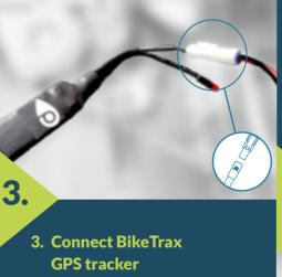
The BikeTrax GPS tracker is coupled with the connection cable.
