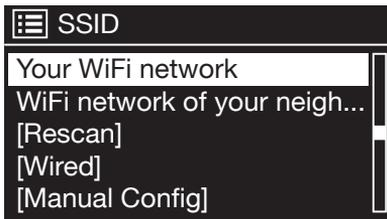
The setup wizard gives you the ability to choose between the cable connection and the wireless WLAN port.
