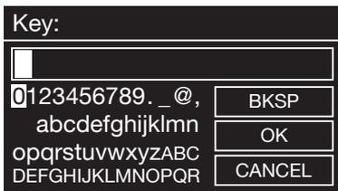
Enter the password for your WLAN router via the navigation dial: turn the dial to select the letters and numbers, and press the dial to confirm the entry. You can find the special characters by scrolling further using the dial.
