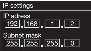
Here you can enter the corresponding values using the navigation dial. To get to large numbers (such as 192) more quickly, turn the dial to the left. To go to the next field, press the dial or the OK button on your remote control.
