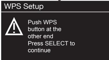
To use this type of connection setup, press the WPS button (PBC) on your router and then “OK” on your iRadio.
