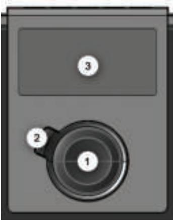
1. *Navigation dial with push function for selection:* Scroll through the menu by turning the dial in the list view. Turning the dial during playback changes the volume. To select a menu item, press the dial once.
