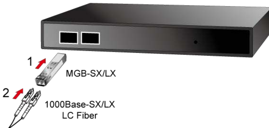
Figure 2-5 Plug in the SFP transceiver
