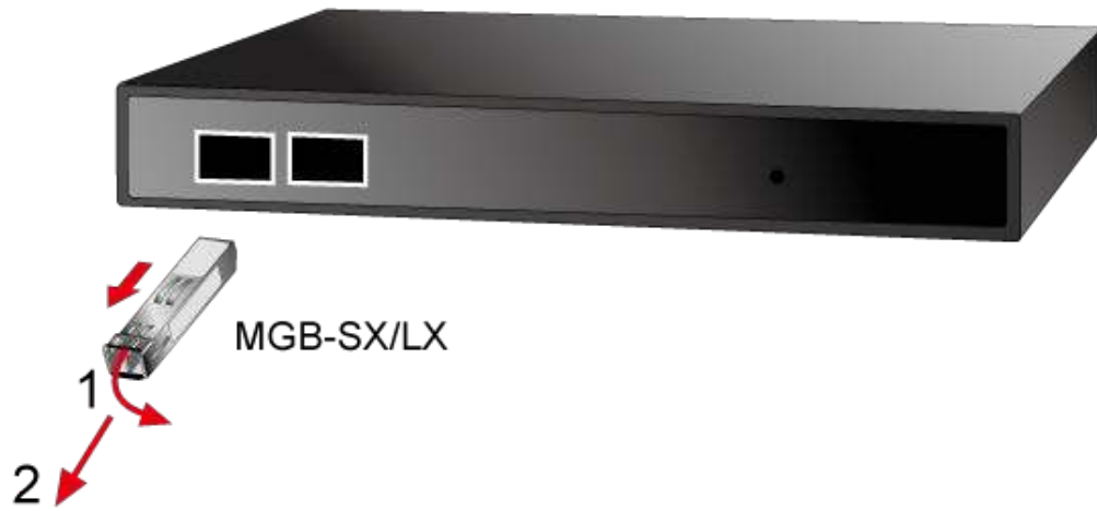
Figure 2-8 How to Pull Out the SFP Transceiver
