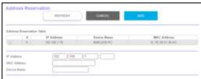
6. In the **IP Address** field, type the IP address to assign to the computer or server.
