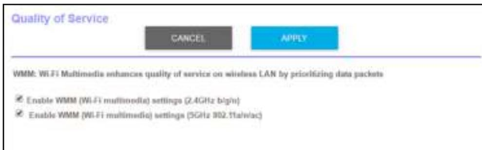
5. Clear the **Enable WMM (Wi-Fi multimedia) settings (2.4 GHz b/g/n)** check box.
