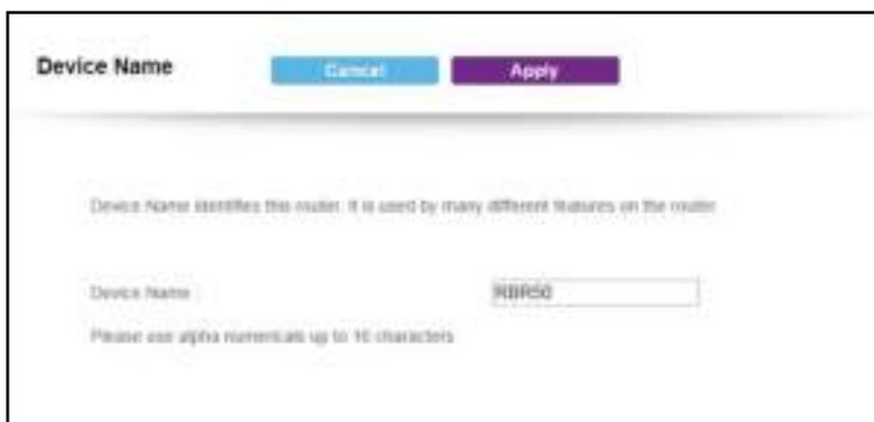
5. In the **Device Name** field, type a new name.
