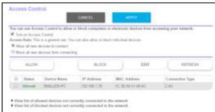
You must select this check box before you can specify an access rule and use the **Allow** and **Block** buttons. When this check box is cleared, all devices are allowed to connect, even if a device is in the blocked list.
