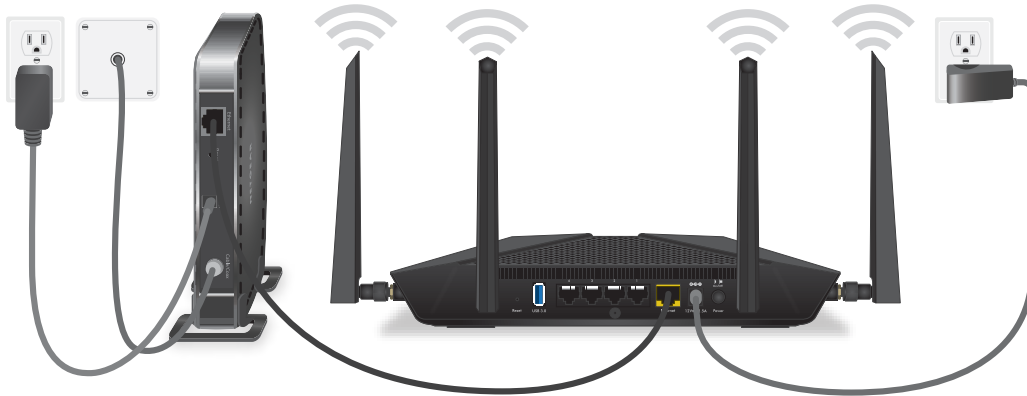
Figure 7. Cable your router
