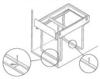
Before permanent attachment to the cabinet base, fit containers and lid and test for ease of opening and container removal. Ensure the unit is clear of door hinges and other obstructions during operation.
