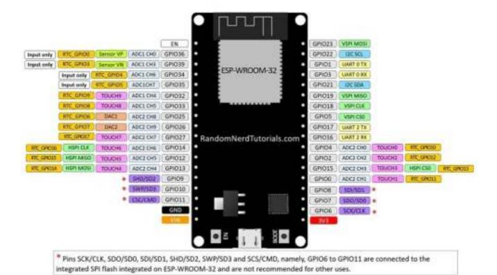
Additionally, there are pins with specific features that make them suitable or not for a specific project. The following table shows what pins are best to use as inputs, outputs and which ones you need to be cautious.
