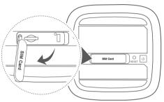
3 Insert the SIM card gently into the SIM card slot in the direction shown in the figure below until it clicks. Then close the SIM card cover.
