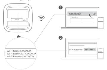
Once the router has connected to a mobile data network, you can connect your computer or mobile phone to the router's Wi-Fi network to access the Internet. Please refer to the label on the bottom of the router for the default Wi-Fi network name (Wi-Fi Name) and password (Wi-Fi Password).
