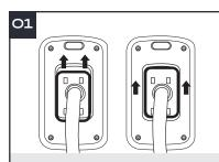
Click the phone holder onto the gooseneck. **NOTE**: you have connected correctly when you hear the "clicking sound."
