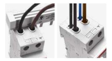
Supply operation is allowed in parallel with busbars and cables (either from top or bottom side) as terminals are composed of two different seats: a front seat for 25 mm2 cables and a back seat for 10 mm<sup>2</sup> busbars.
