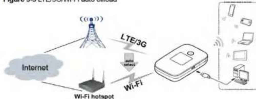
Figure 3-3 LTE/3G/Wi-Fi auto offload
