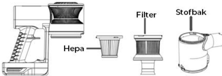
5. Replace the HEPA filter every 3 months. The filters can be ordered via the QR below.
