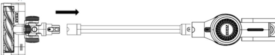
Attach the electric floor brush to the aluminum tube until it clicks into the correct position.
