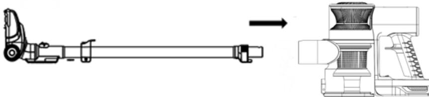
Attach the tube to the connection port of the main device.
