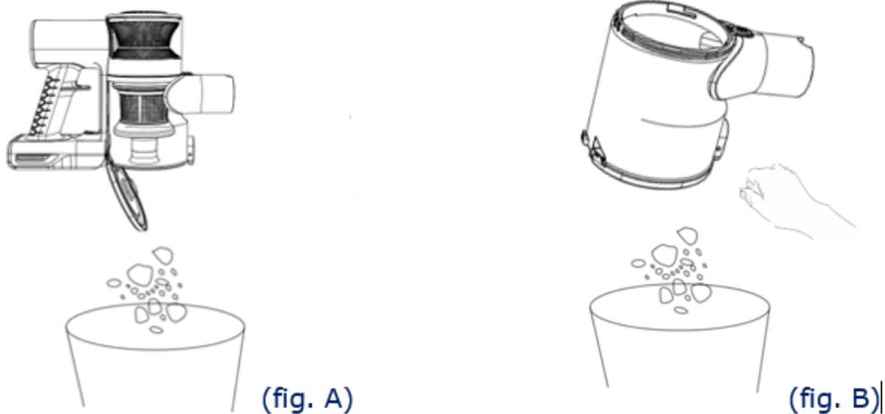
4. Remove the filter assembly: filter, Hepa, dust container.
