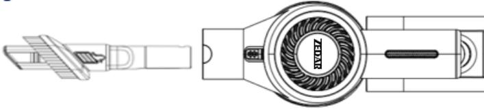
Attach the crevice tool to the main unit until it clicks into the correct position.
