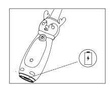
4. Please pay attention to the status of the battery indicator light, flashing The battery is low and needs to be charged.
