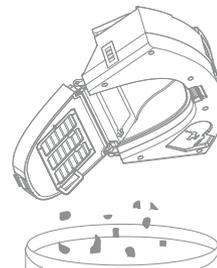
4. Take out the high efficient filter HEPA and the primary filter, tap the high efficient filter HEPA to remove dust
