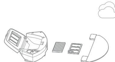
**!** Before installing the filters, make sure that the high efficient filter HEPA and the primary filter are dry.
