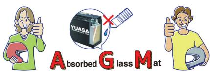
AGM separators retain the electrolyte and help the internal gas absorption to negative plates. This makes the battery require no refilling and realize maintenance free.
