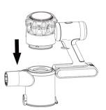
3. Take out the HEPA from the HEPA cover and wash the HEPA filter and HEPA cover with cold water. Install them on the vacuum cleaner when they are completely dry. Do not dry with a hair dryer.
