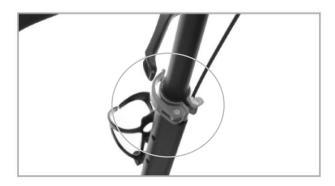
By opening the quick release, you can adjust the steering to a comfortable height. Make sure the knob snaps into a hole in the steering column. After adjustment, close the quick release.
