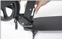
Open the rapid tightening lever and press the folding button to unfold the Scooter.
