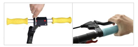
Adjust the lock to tight the T-bar without space, hold the brake handle to restore the brake line.
