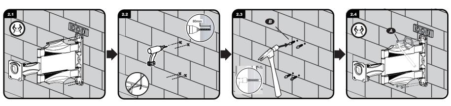
Attach mount to wall (Solid Concrete wall)
