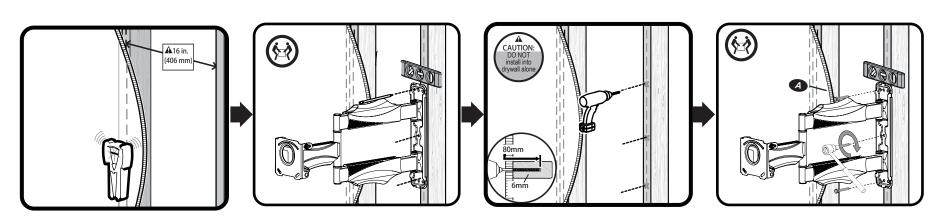
Attach mount to wall (Wood Stud wall)
