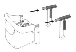
1. Insert two iron pipes of the fixing bracket into the tube of the chair through two round holes.
