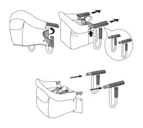
1. Unzip the lower support arm cover over the support arms. Loosen the clamps by rotating them clockwise. Remove hook-on chair by pulling it away from the table.
