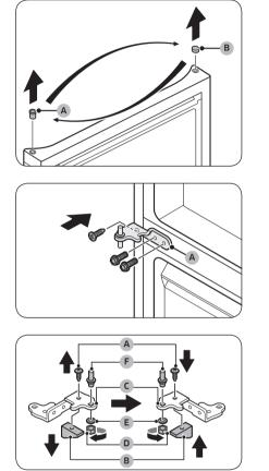
**14.**On the top of the freezer door, switch the position of the grommet (A) and the grommet cover (B).
