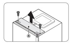
With the fridge door closed, use a Phillips screwdriver to remove the screws fastening the top cover (A). ( )
