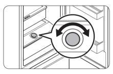
Humidity Fresh+ allows you to adjust the humidity. Turn the control dial left or right to adjust the humidity as you desire.
