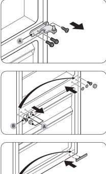
**9.** Use a Phillips screwdriver and socket wrench (10 mm) to remove the screws fastening the **middle hinge (A)**.
