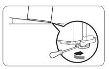
To adjust the height of the left side: Insert a flat-head screwdriver into the leveller of the front left leg. Turn the leveller clockwise to raise, or turn it anticlockwise to lower.
