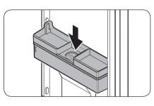
**3.** Reinsert the water tank and close the door. Make sure the water outlet of the water tank faces forward.
