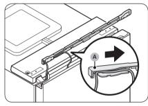
**37.**Put the provided **top-right door cover** (A) on the opposite side of the door hinge.
