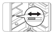
Optimal Fresh+ drawer allows you to divide the area into two separated zones using the Flex Divider.
