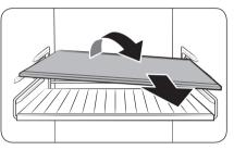
1. Pull out the shelf (or Rack & Shelf) a little. Then, while lifting the rear side, pull out.
