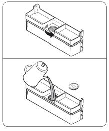
1. Hold the handgrips on both sides of the water tank and lift up to remove.
