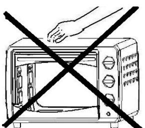
Be careful! Not to burn yourself during use or immediately after use. The metal parts and glass window of the door become extremely hot during use. Be careful not to touch them when opening and closing the door.
