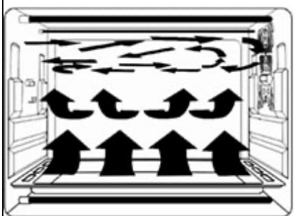
Featured with a special convection function, strong and absolute cycling airflow by making the heating more complete. Original flavor can be kept.
