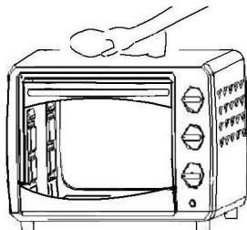
When cleaning, wash the interior and exterior surface, bake tray, wire rack and tray handle with soft cotton (or sponge) with neutral cleaner. Then wash with clean water. Do not use hard brush or any others to wash, so as not to scrape the interior surface of the oven, and to protector of the bake tray, the wire rack and the tray handle.
