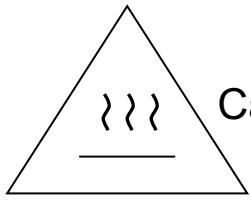
Caution: The temperature of the accessible surface may be high when the appliance is operating.
