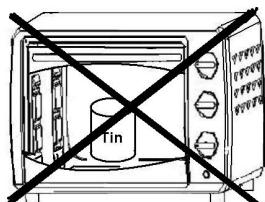
Any bottled or tinned food can not be heated directly as prevent the bottle or tin would be broken out and scald the person.
