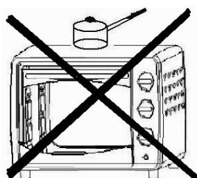
Do not put anything on the oven while using it, the heat could cause deformation, cracking, etc.
