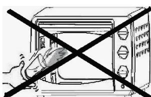
When hot, do not apply water to the glass window. It may cause the glass to break.
