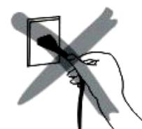
When unplugging the cord, always take hold of the plug itself. Never pull on the cord. Doing so could break the wires inside the cord.
