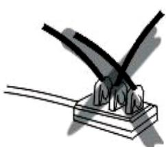
AC power must be taken from a properly wired outlet. Insert the plug completely into the socket. If it is not, it could become abnormally hot. Do not use an electric light outlet. Never connect multiple plugs to the same outlet.
