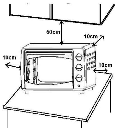
If the oven is positioned to close to a wall, the wall will be burned or stained. Be sure the curtain, etc. are not in contact with the body. Do not put anything between the bottom of the body and the surface on which it is set, an object so placed could be burned.
