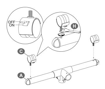
Insert the pole into the bottom  $\,$  of the plastic parts, and then tighten the screws.
