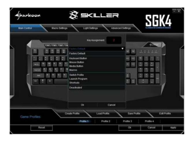
In the Main Control, the individual keys can be reassigned or allocated functions. The Esc key, P1 to P4, L1 to L4, F1 to F12, the Windows key, the W key, the arrow keys and the SKILLER key cannot be reassigned.
