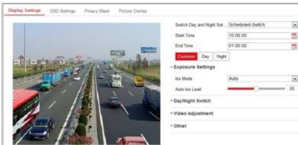
Figure 9-5 Day/Night Scheduled-Switch Configuration Interface
