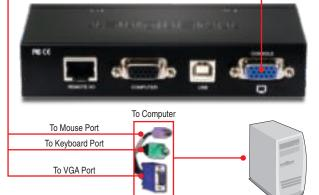
9. Connect a Cat.5/5e/6 Ethernet cable from the Ethernet port on the Transmitter (local device) to the Ethernet port on the Receiver (remote device).
