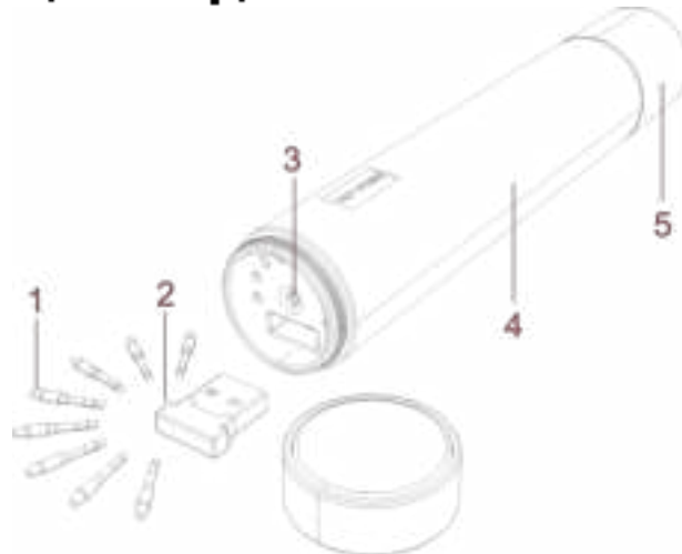
Image 2-2 Pen Case, Pen stand, Pen tip, USB receiver and Pen clip hole
