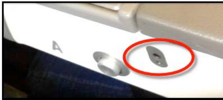
Figure 1.9 – Input Jacks on an Airplane Seat (Armrest)
