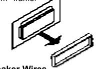
Insert the keys supplied with the old unit into both sides of the unit as shown in figure below until they click. Pull to remove the old unit from the dashboard.
