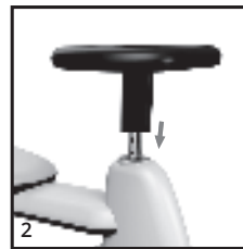
Figure 2: Install the steering wheel (part 2) into the hole of the car body (part 1).
