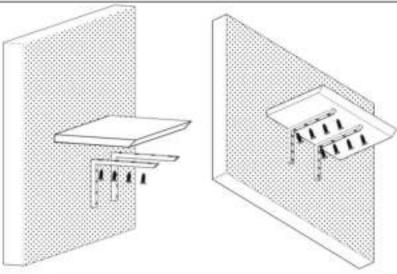
FIX THE LEGS COMING TOGETHER WITH THE PRO-DUCT TO THE TABLE PLATE FROM THE MARKED POINTS
