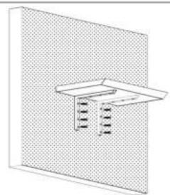
MOUNT THE TABLE PLATE WITH FIXED LEGS TO BE FLAT ON THE WALL WITH THE HELP OF ANCHORS.
