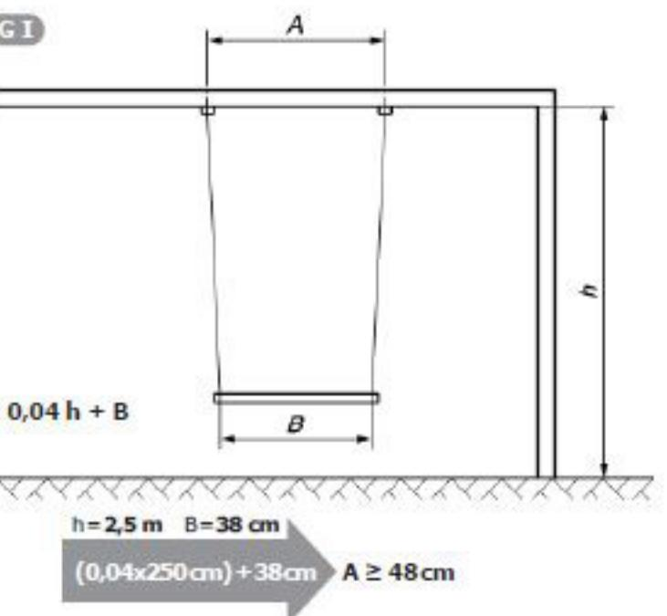
A distance between the suspension points along the crossbeam.
