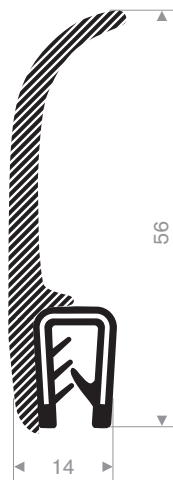
245.00.876 pvc + mosrubber klembereik 1-3 mm
