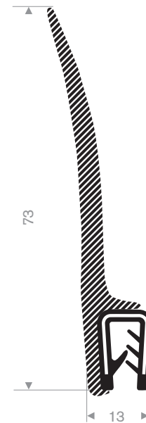
245.00.877 pvc + mosrubber klembereik 1-2 mm
