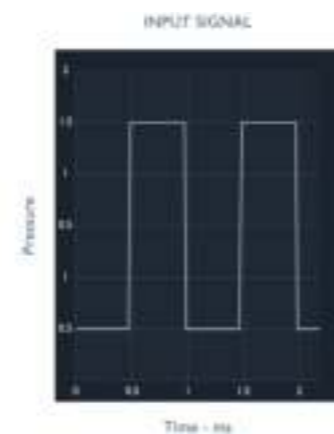
Figure 56 Input signal - 1kHz square wave
