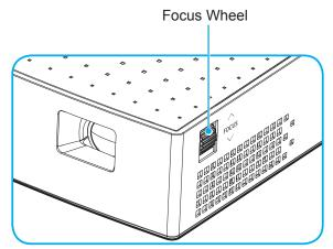
Note: The projector will focus at a distance of 0.6m to 1.9m.
