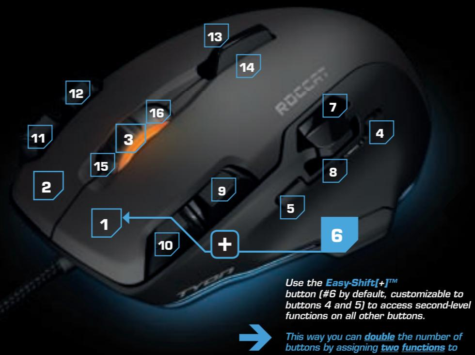
Use the Easy-Shift[+]™ button (#6 by default, customizable to buttons 4 and 5) to access second-level functions on all other buttons.
