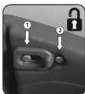
Latch in permanent "unlocked" position; install (2)  $\frac{1}{2}$ " (1,27) screw.
